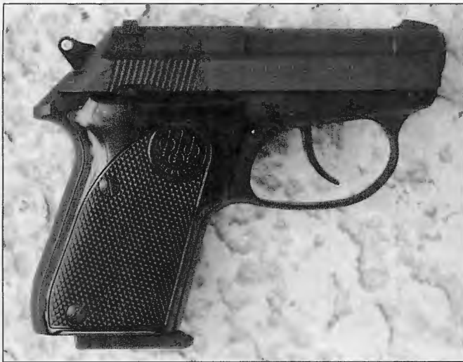
Beretta Tomcat, right-side view — note trigger mechanism's external transfer bar protruding along the top of the frame in front of the grip panel.
